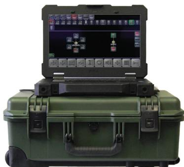
The Codan RIOS provides interoperability between a range of communications devices, including radios, smartphones and computers, enabling a fully integrated communications network from anywhere in the world. The Codan RIOS is the solution for enabling users with different vendor devices to seamlessly communicate across any platform.
